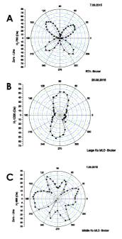
Figure 1. Angular in-plane dependence of the resonance field measured by ferromagnetic resonance (FMR).
